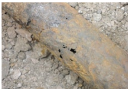
This picture shows an 8" steel gas main operating at pressures between 75mbar and 2bar, showing severe signs of corrosion. In this instance the main has suffered multiple through-wall corrosion events.
