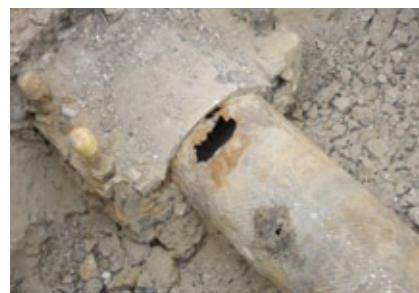
This picture shows a 6" steel gas main that had a repair clamp fitted in the past. As can be seen the gas main is in a continuing state of deterioration resulting a large through-wall corrosion incident alongside the pipe clamp.
