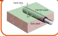
of water samples when present. The water's PH level will be tested on site to determine the acidity level which indicates the severity of the pipeline's environment. This visual assessment and water analysis will provide SGN with a clear indication of corrosion without the need to excavate, eliminating the interference and informing us of any future actions to take.
