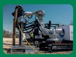
Testing has progressed with mounting the excavator head onto the robotic arm and using test beds with varying soil types including compacted hard clay. The ability to utilise the robotic arm for excavation has improved the precision in excavation operation. More testing is required to improve on the system and the process to make the excavator more robust and effective.
