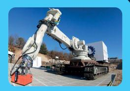
Using our mock roadway which represents a typical utility highway complete with mixed material pipeline and ducts, the team have commenced the testing of the sensor module. The results have been positive with a high accuracy of detection at various depths. More testing is to be conducted to improve accuracy of detection within different soil types.
