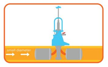
This NIA project (NIA\_SGN0093) allows use of an existing process and equipment by developing an appropriate electrofusion fitting to allow connection to the PE main and installation of the existing under pressure drilling machine and bag off equipment. The new fitting will be specifically designed to be compatible with not only the bag off equipment but will also allow use of the Synthocam 3 camera system and the I-branch water extraction tool.
