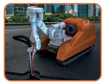
As RRES will take up less space than conventional methods and remove the operator from the hazardous excavation zone, the system will have significant financial, safety and environmental benefits. Furthermore, since RRES will provide a complete end to end solution,
