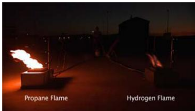
Figure 8 Comparison of propane and hydrogen flames at night (from [5])
