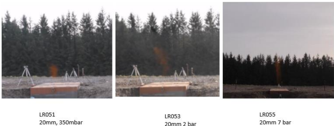
Figure 1 Large scale hydrogen releases performed as part of the H21 test programme
