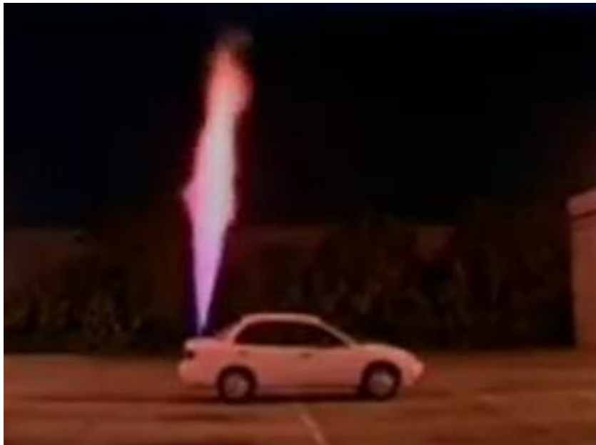
Figure 10 Ignited release from pressure relief system on a hydrogen fuelled car [9]
