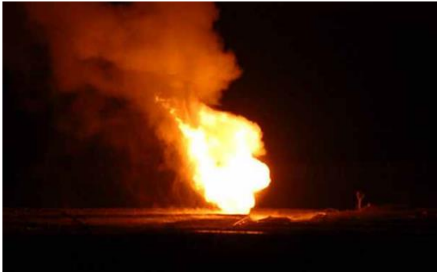
Figure 2 Rupture test of a buried 6" pipeline operating at 60 bar
