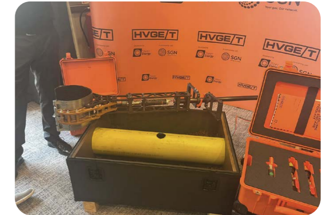
The High Volume Gas Escape Toolbox is just one innovative solution we’re using to respond to leaks in our network.
