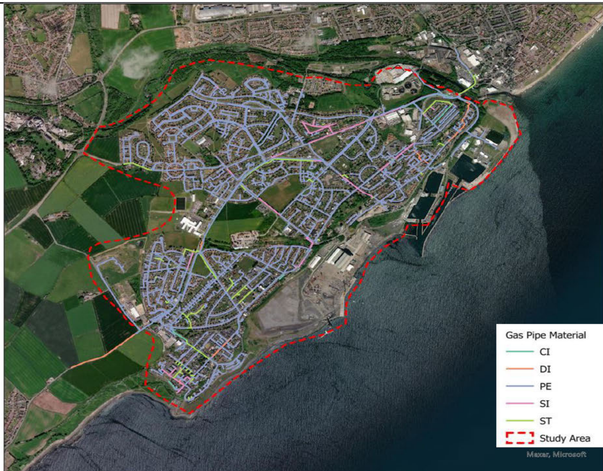
Figure 26 Network map showing the composition of the current gas pipe material within the study area. CI = cast iron 2.1%, DI = ductile iron 1.5%, PE = polyethylene 85.1%, SI = spun iron 6.3%, ST = steel 5%
