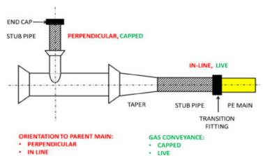
There are various components that may be found in the construction of a stub, the configuration differs on every occasion but can be seen in figure 1 above and generalised by:
