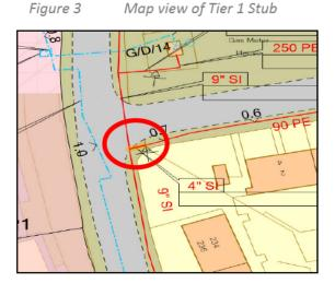
highlighted in green, of 2.2m and a maximum stub length of 2.0m, highlighted in red. Therefore, using remediation techniques from table 2 above we have the options of either shortening the stub to 2.0m or less, inserting the Sealback method, or carrying out a full stub using the parent main cut-out.
