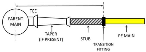
Figure 2 shows the most common perpendicular arrangement and indicates how the overall length of the stub is measured, known as the digitised length. It is taken from the middle of the parent main to the last non-polyethylene component.
