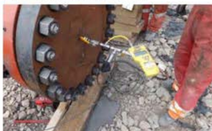
Figure 33: Pressure testing of horizontal tee.
