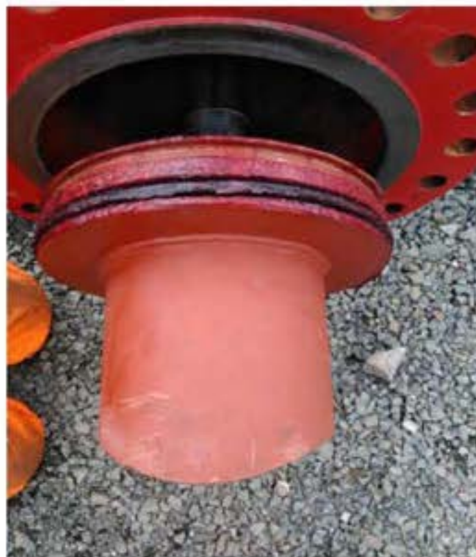
Figure 36: Swarf accumulation in split tee.
