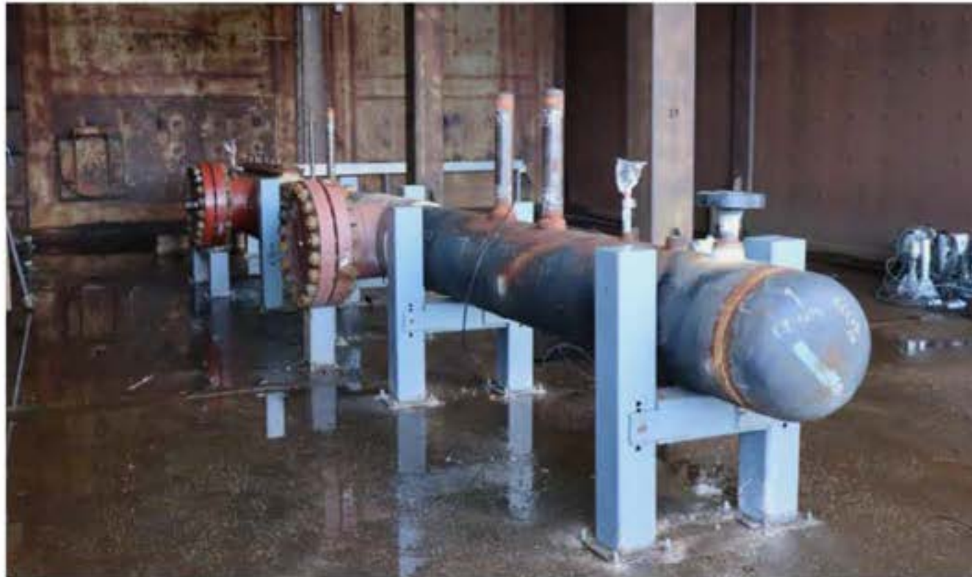
Figure 85: Fatigue vessel incorporating grouted and welded tee connections.
