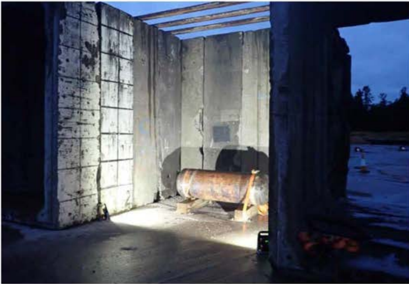
Figure 81: Burst test vessel pre-test.
