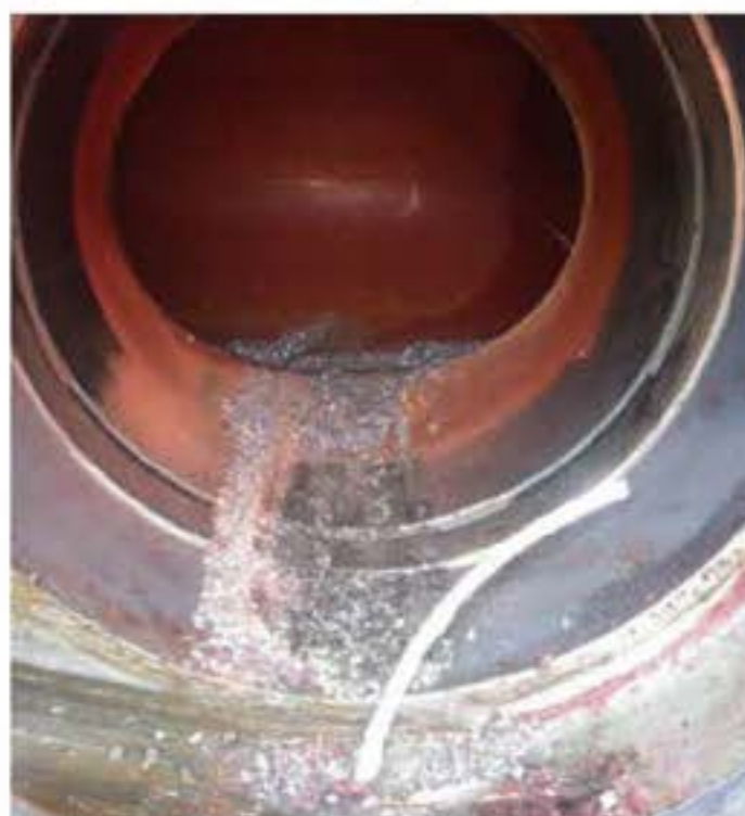
Figure 36: Swarf accumulation in split tee.
