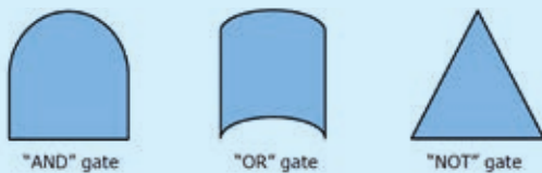
Fig. 62 Fault tree gates
