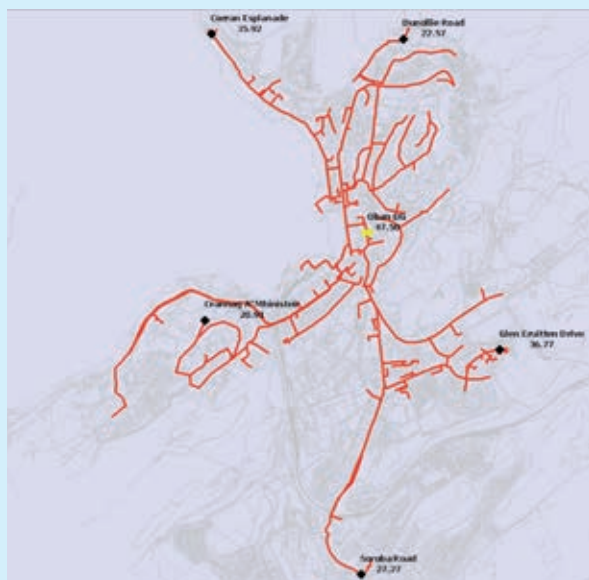
Fig. 72 Oban network pressure reduction on trial gas
