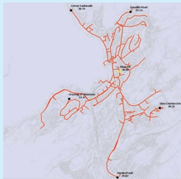
Fig. 71 Oban network pressures on trial gas
