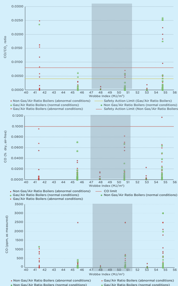
Fig. 28 Laboratory test results – boilers
