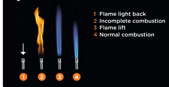
Fig. 2 Gas flame effects
