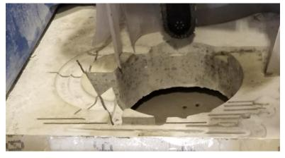
Figure 4 Chainsaw cut - circle, triangle and straight lines for testing
