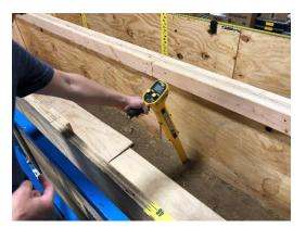
Figure 12 – Magnetonmeter Soil Box Test
