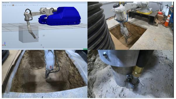
Figure 7 - Excavator head mounted at the end of the robotic arm
